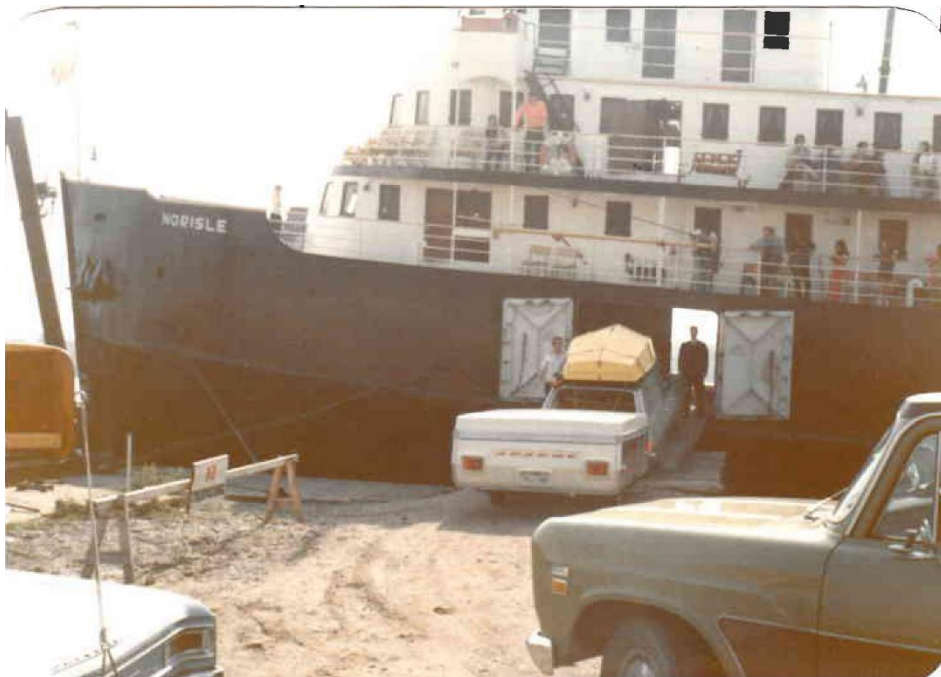
The Norisle was a side loader and cars would drive on or be driven on and parked on the upper car deck or taken down to the lower car deck by an elevator. This picture is c1973.
